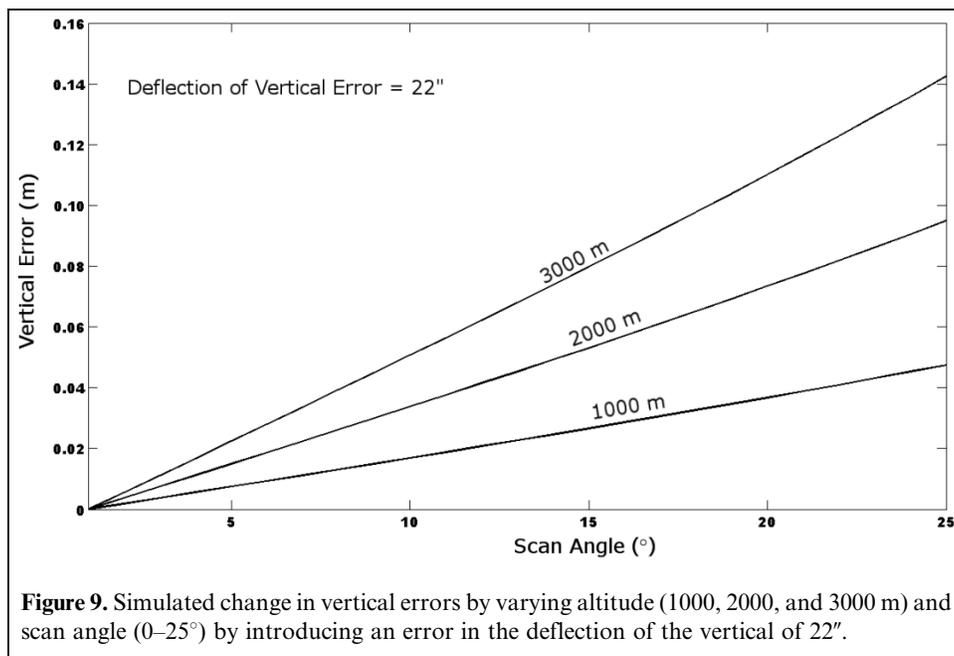
**Figure 9.** Simulated change in vertical errors by varying altitude (1000, 2000, and 3000 m) and scan angle (0–25°) by introducing an error in the deflection of the vertical of 22".
