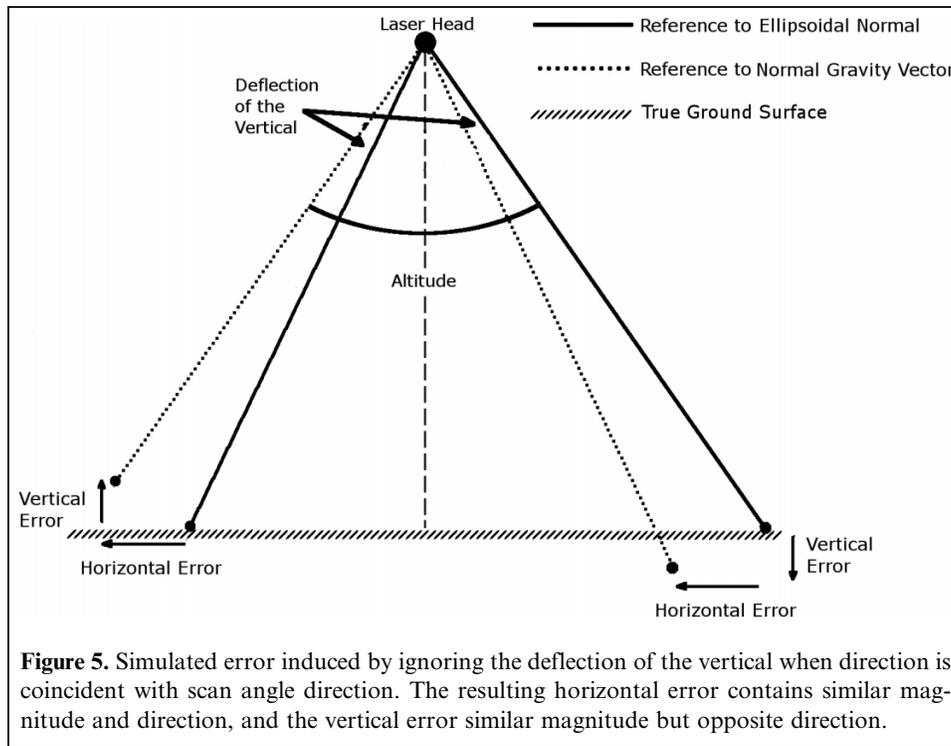
and sign, whereas the vertical error is equal in magnitude but opposite in sign. This creates swath edges that are vertically separated by twice the induced vertical error.
