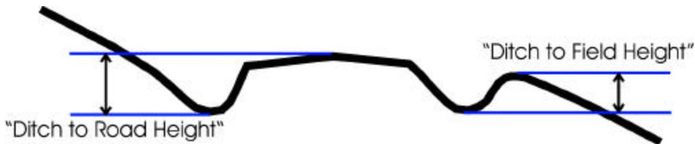
Figure 5. Road cross-section ditch-to-field and ditch-to-road heights.
