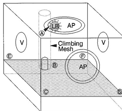
**FIG. 1.** To elevate their body temperature by basking, nymphs had to climb a plastic mesh (8-cm diameter  $\times$  28-cm high) toward a heat source (25-W incandescent light bulb; LB) in a aluminum cage (40  $\times$  40  $\times$  30 cm). The cage was equipped with a perforated metal floor and a clear Plexiglas top and front. Air flow was enhanced by mesh vents (V) and access ports (AP), and temperatures were monitored at points A to F.
