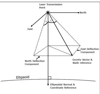
**Figure 3.** Effect of deflection of the vertical components applied to lidar scenario. The scan angle and IMU observations are referenced to the gravity vector, and the coordinates are referenced to the ellipsoidal normal, resulting in an angular shift of observed features. Adapted from Figure 6.9 of Jekeli (2001).
