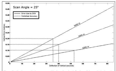
**Figure 7.** Absolute vertical error caused by ignoring the deflection of the vertical when the direction is coincident with scan angle direction. Errors are displayed for separate altitudes of 1000, 2000, and 3000 m. Published accuracy for each altitude is represented by the horizontal broken lines and correlated with deflection of the vertical magnitude.
