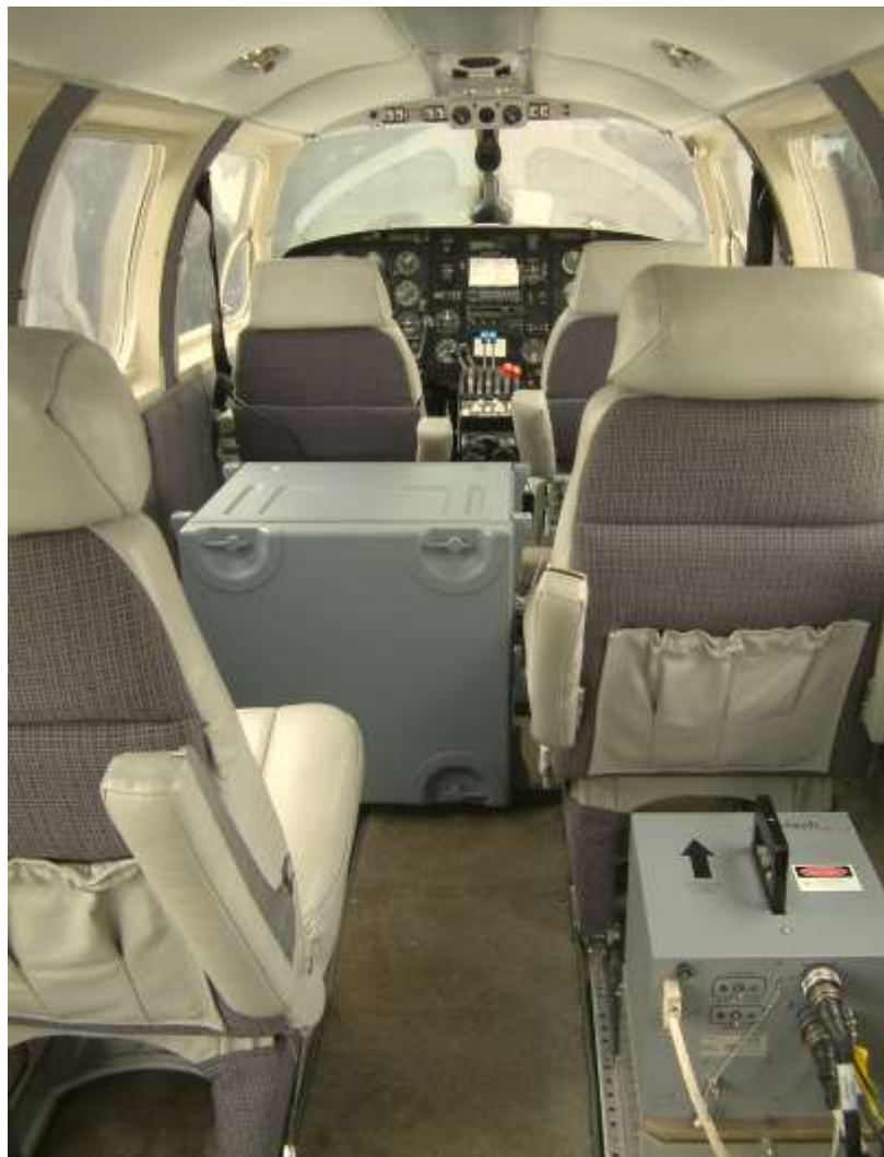
Figure 8. The interior of the survey plane illustrating the locations of the sensor head (rear starboard side) and the control rack (centre port side). The only difference between this configuration and that used during the boreal forest missions, was that a camera control rack was mounted above the ALTM rack plus the RGB digital camera was mounted ahead of the ALTM sensor head.
