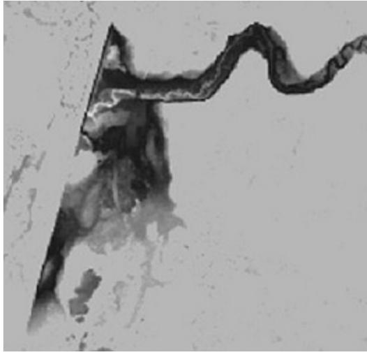
**Figure 9:** The fill command is useful for finding locations that act suspiciously. This is a road blocking a small stream a culvert needs to be added to allow flow across the road.
