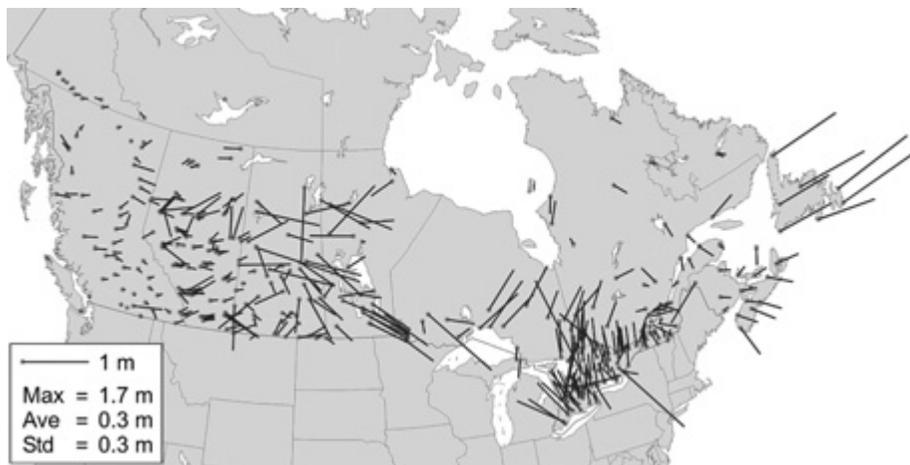
**Figure 2:** Errors in NAD83(Original) as revealed by high accuracy GPS observations in NAD83(CSRS).
