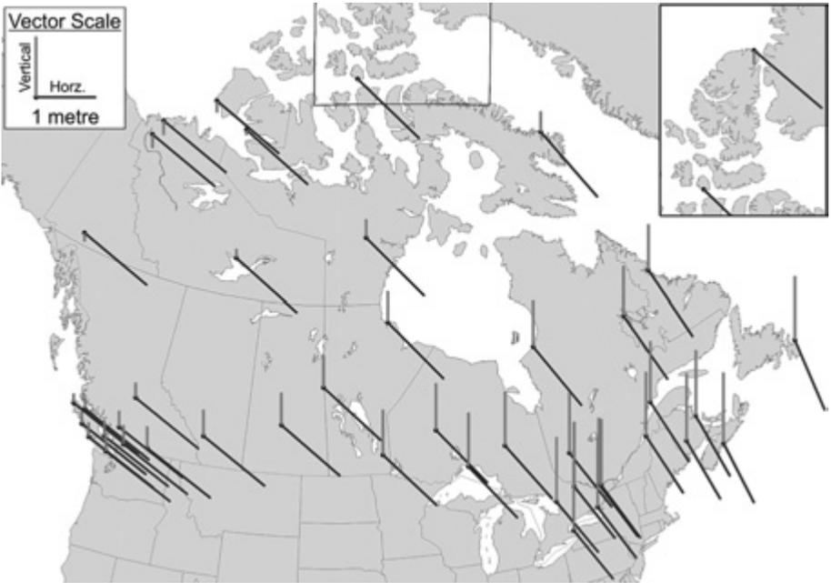
**Figure 6:** Horizontal and vertical differences between NAD83(CSRS) and WGS84 in the sense NAD83(CSRS) minus WGS84.
