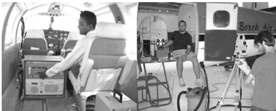
**Figure 5:** Installation of an Optech ALTM 3100. Left installed and ready to go inside a Piper Navajo. At right surveying in the GPS antenna lever arm offset during installation into a Twin Otter. Note survey prism located over sensor reference point.
