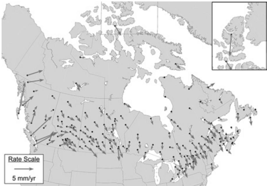
**Figure 7:** GPS horizontal velocities from repeated high accuracy GPS observations with respect to the NNR-NUVEL-1A plate motion estimate for North America. The coherent pattern reveals a bias in NNR-NUVEL-1A of about 2 mm/y.
