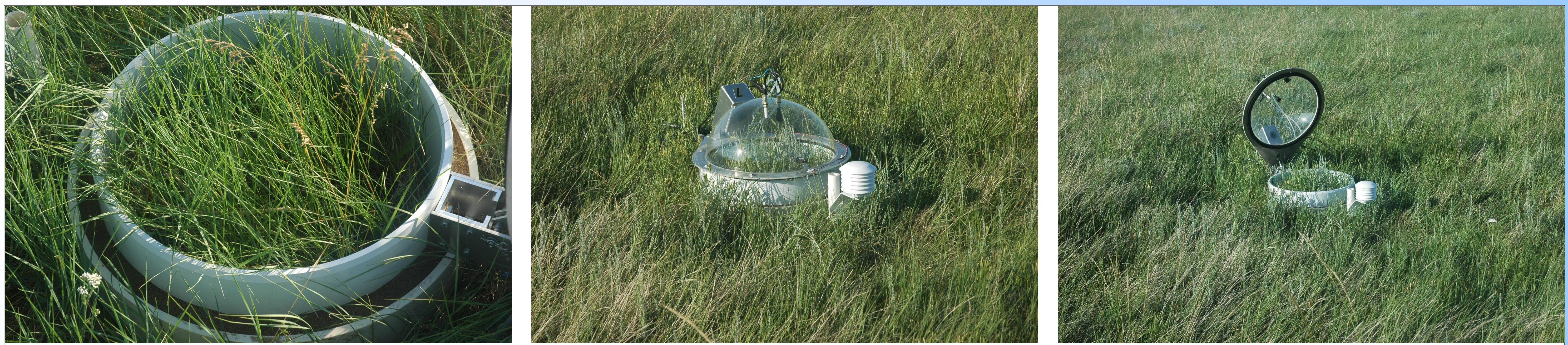
Automatic Net Ecosystem CO 2 Exchange Chambers with Sand-Ring Collar
