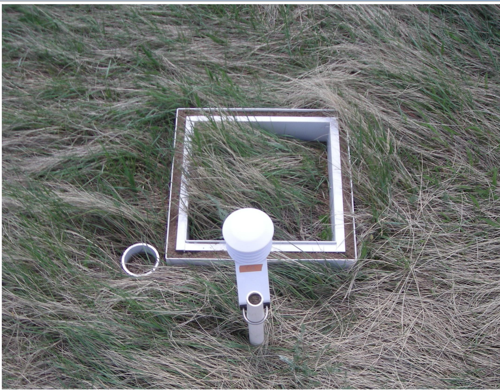
System for Chamber Measurements of Ecosystem CO 2 Exchange
