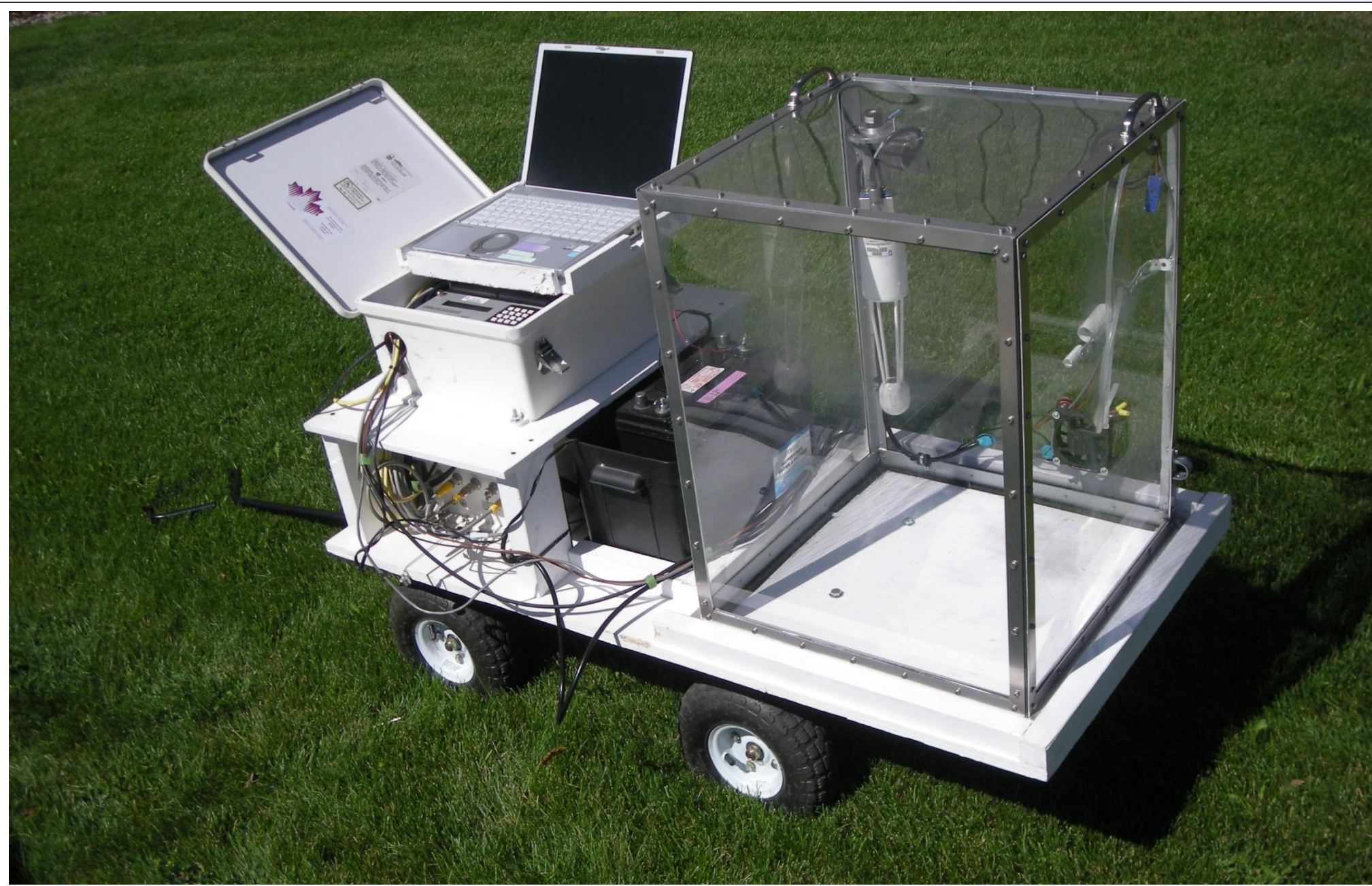
System for Chamber Measurements of Ecosystem CO 2 Exchange
