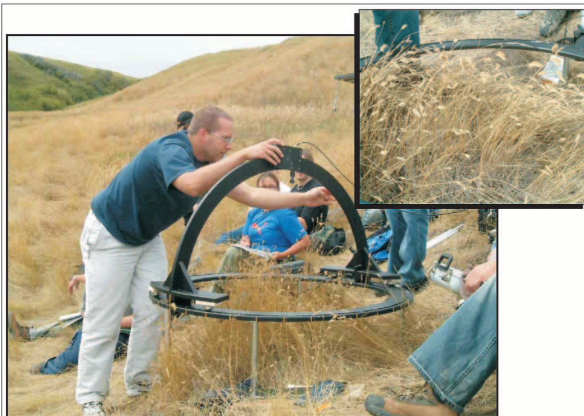
Figure 4. Field use of ULGS goniometer on a sloped surface at grassland meteorological station located in the coulees of the Oldman River valley in the southern portion of the University of Lethbridge campus. The inset is a close-up of the crested wheatgrass target (oblique view).
