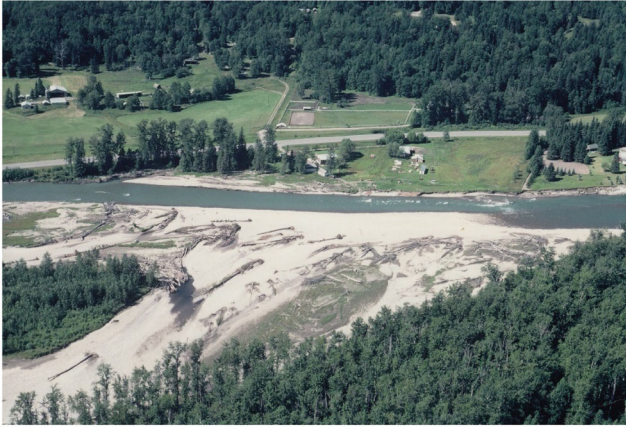
Figure 3. An oblique aerial view of major erosion Site 5 (49°24 40″N: 115°05 00″W) in which the Elk River avulsed and moved from a left bend (lower left barren zone) to the right, through a prior grassland hayfield. The river swept right until it reached the Highway 3 roadway that was subsequently armoured with large boulders.
