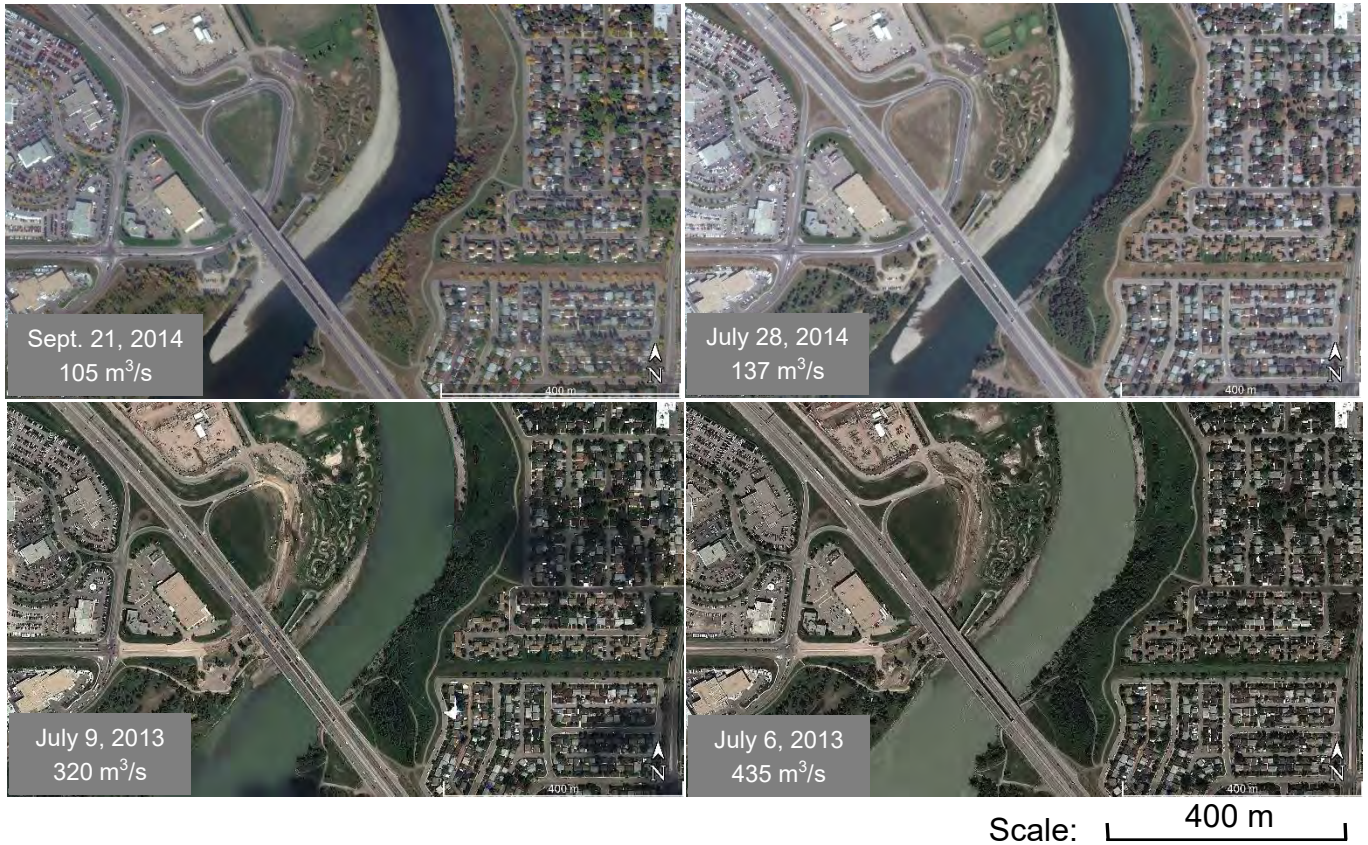
Figure 31. Post-flood aerial photographs of Glenmore Trail Bar in the Bow displaying the inundations at different river discharges that were used to project vegetation colonization patterns.
