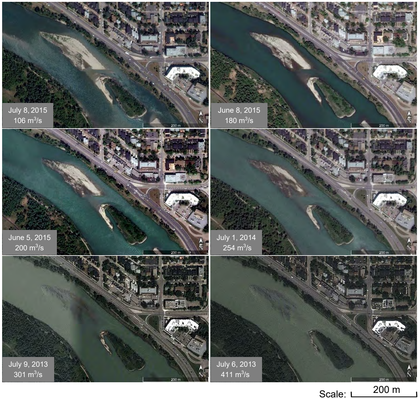
Figure 13. Post-flood aerial photographs of Shrub Island in the Bow River, which were used to coordinate inundation discharges for that study site.
