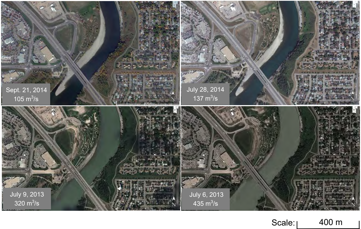
Figure 69. Post-flood aerial photographs of Glenmore Trail Bar, displaying the inundations at different river discharges that were used to project vegetation colonization patterns.
