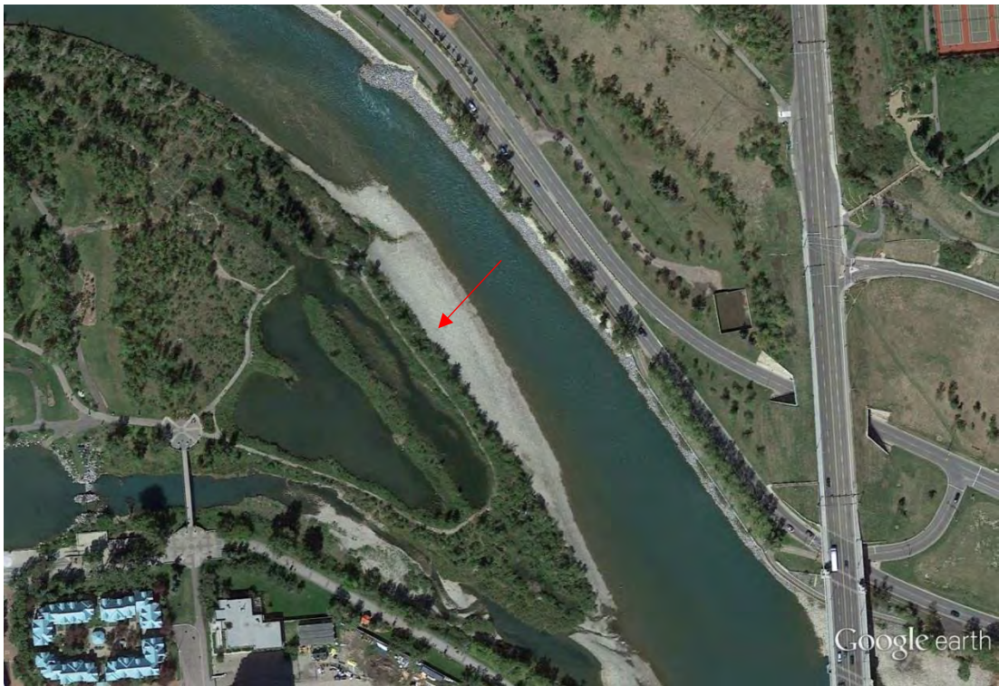
Figure 56. Aerial photographs of the zone displayed in the Figure 54 photograph, illustrating the transition from the barren gravel bar to the band of perennial riparian vegetation. The red arrows indicate the direction of the ground level photo. The upper photo displays the river inundation at around the Q_2 , or average annual peak discharge, supporting the association between this and the Ordinary High Water Line (OHWL).
