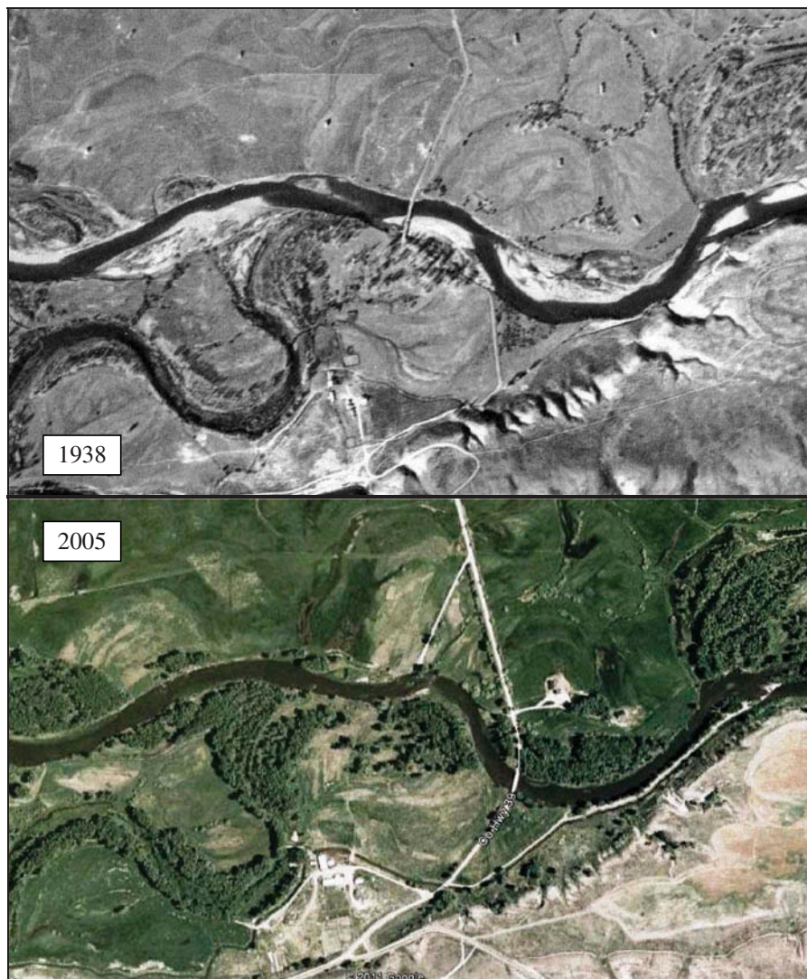
Fig. 5 Aerial photographs of the Colorado River above Troublesome Creek (Lat. 40.055°N, Long. 106.29°W), comparing pre-dam 1938 (23 October) to post-dam 2005 (17 June). The active channel decreased on average 63% during this period, and point bars and islands have been colonized by narrowleaf cottonwood and willows.
