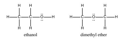
Both molecules are polar; however, ethanol molecules are able to hydrogen bond with other ethanol molecules (while dimethyl ether molecules cannot hydrogen bond with each other). As such, the intermolecular forces in liquid ethanol are stronger overall than those in liquid dimethyl ether and it has a higher boiling point.
