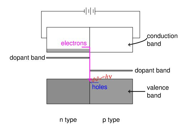
The basis of an LED is an n-p junction (diode). Electrons are fed into the n side of the junction by an external power source, shown here as a battery. The electrons naturally tend to migrate to the p side of the junction due to the relatively empty conduction band on that side. However, LEDs are engineered so that, right at the junction, there is a high probability that electrons will combine with holes in the valence band of the p-type semiconductor.
